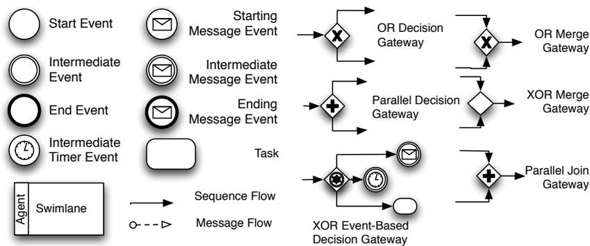
Fig. 4. A core subset of BPMN elements
